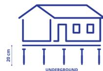
Extremely flexible, screw foundations are **ideal for areas with restricted access and inclined deployment areas**. It does not need concrete foundations.
