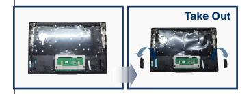
Separate 14: Cut (Extrusion Coat × 12) to take out the object.
