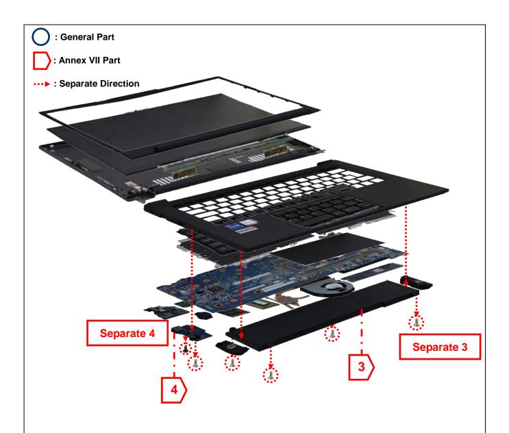
Separate 3: Unscrew (Cross  $\times$  4) all joints to take out the part 3.
