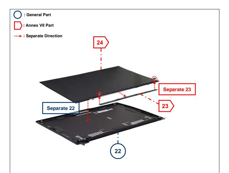
Separate 22: Pry (Glued Joint × 1) to take out the part 22, and rip (Glued Joint × 1) the label.
