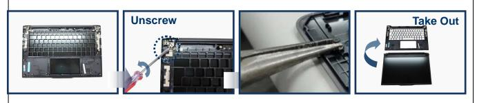
Separate 19: Pry (Snap Fit × 28) to take out the part 19.
