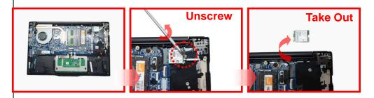
Separate 8: Unscrew (Cross  $\times$  3) all joints to take out the part 8.
