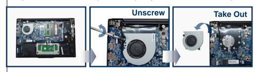
Separate 12: Unscrew (Cross × 5) all joints to take out the part 12.
