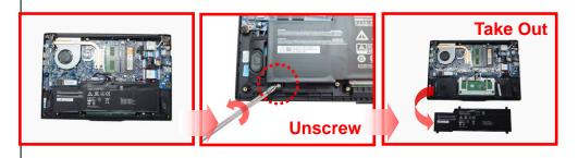
Separate 4: Unscrew (Cross  $\times$  2) all joints to take out the part 4.
