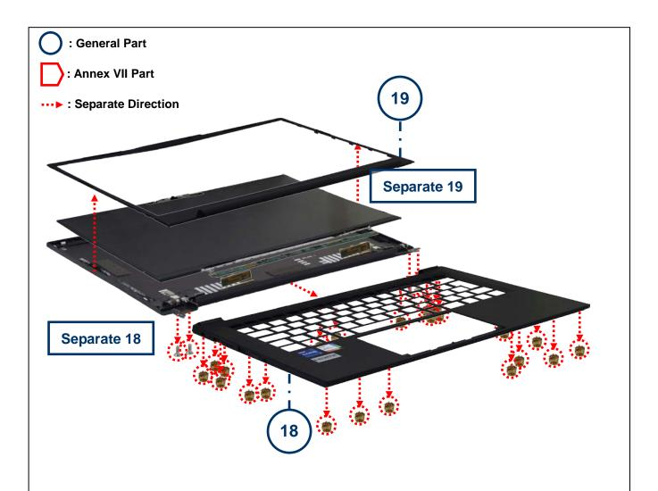
Separate 18: Unscrew (Cross  $\times$  4 & Nut  $\times$  22) all joints to take out the part 18.
