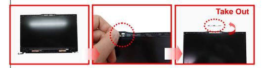
Separate 21: Pull out (Wire Connection × 4) the part 21.
