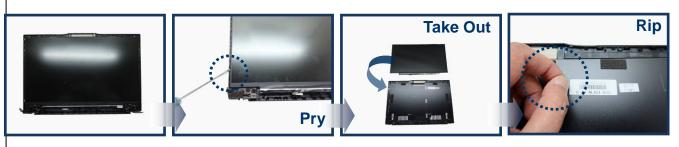
Separate 23: Unscrew (Cross  $\times$  2) all joints to take out the part 23 from 24.
