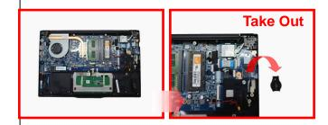
Separate 6: Unscrew (Cross × 2) all joints to take out the part 6.
