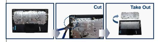
Separate 17: Cut (Extrusion Coat × 58) to take out the part 17.
