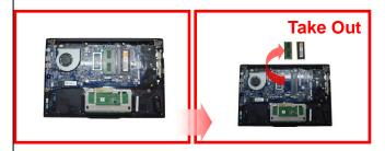
Separate 10: Unscrew (Cross  $\times$  1) the joint to take out part 10.
