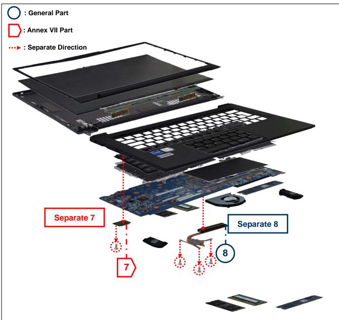
Separate 7: Unscrew (Cross  $\times$  1) the joint to take out the part 7.
