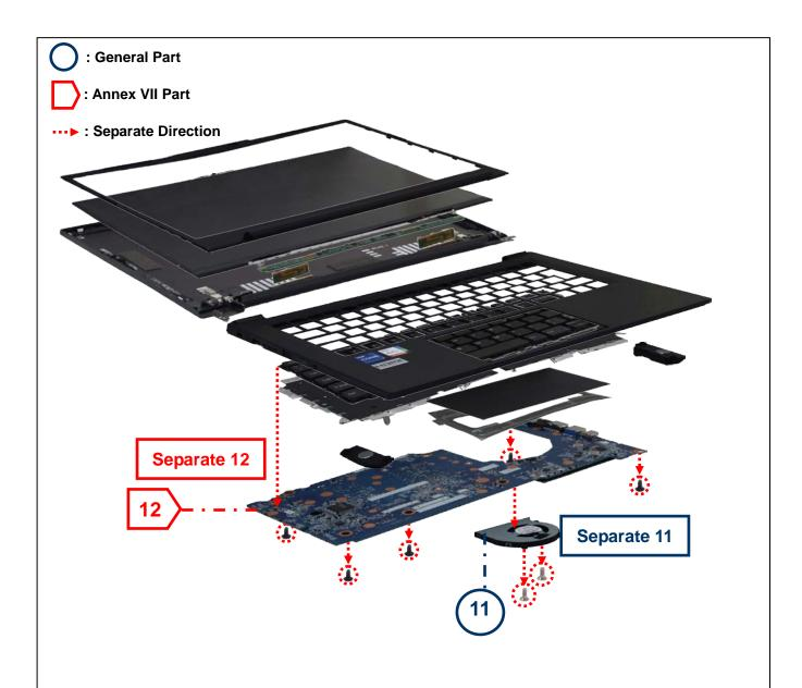
Separate 11: Unscrew (Cross × 2) all joints to take out the part 11.
