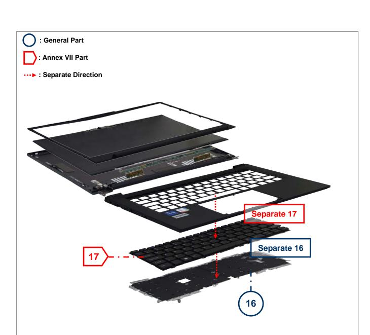
Separate 16: Cut (Extrusion Coat × 34) to take out the part 16.
