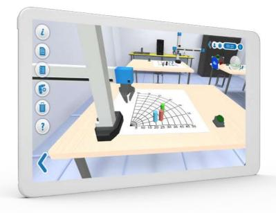
Students can explore different ways to program robots using a graphic block language, block language to solve challenges dealing with manipulation, control, storage and parts relocation.
